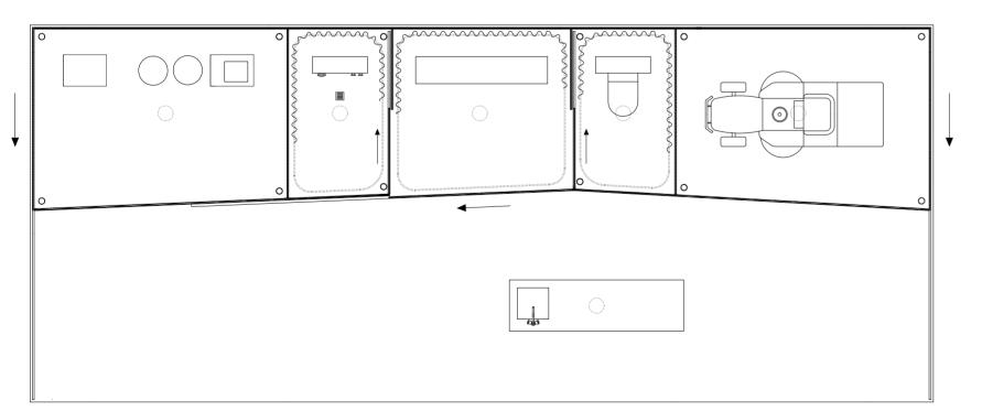
This pavilion combines space for the lawnmower, pool equipment, storage space, shower, WC, changing facilities and a bar. The pavilion can be opened out by means of three large sliding doors. The equipment is stored behind the glass façade, the lines and edges of which dissolve into white dots and which reflects the garden vegetation. In the WC, shower, and changing room areas, curtains are used to flexibly provide as much privacy as desired.
